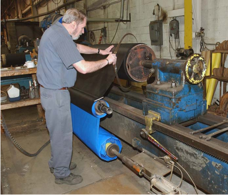
Roll builder Don Miller checks the diameter of a roll he's building at Eagle Rubber.
