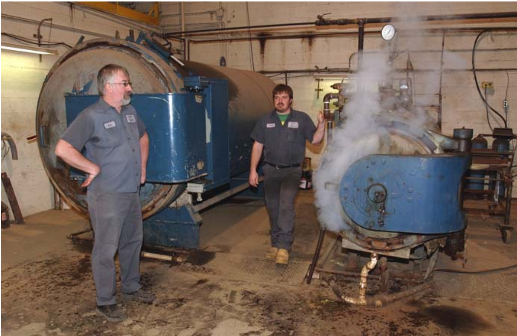
Eagle Rubber roll builders, from left, Don Neff and George Lill prepare an autoclave to cure rubber products
